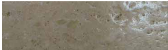
Food stains on stone surface with SurfaPaint Stone Varnish WB. 24 hours after, the stains were removed with water and paper
