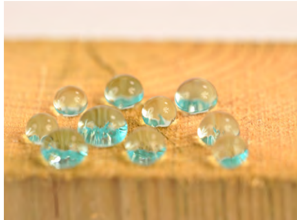
Picture 55 - Application of SurfaPore W on the most absorptive pine wood cut
