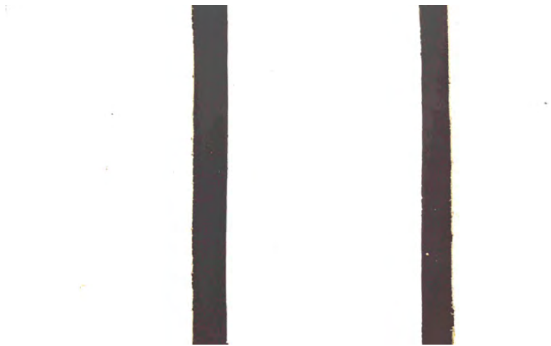
Picture 79 – 36 months exposure sample in the humid and hot environment of Florida. Any competing coating is developing fungi and mould growth, due to the dampness the coating is absorbing (Q-Lab testing ground, Exposure: 45° – South FL, USA)
