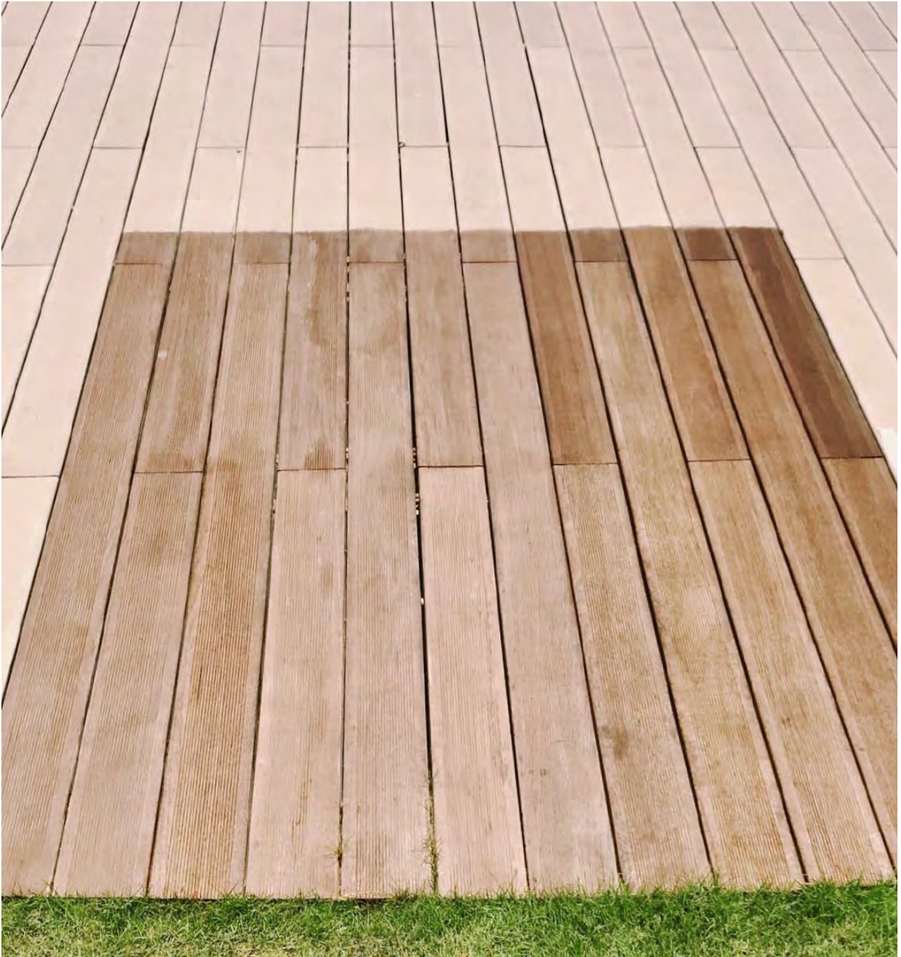
Picture 41 - Application of a single SurfaPaint HDO coat on wooden composite deck flooring. Upper right application corner has been treated with an extra SurfaPaint HDO coat. Photo is taken 12 months after application on a sample applied next to coastline area and subjected to desert heat/irradiation.
