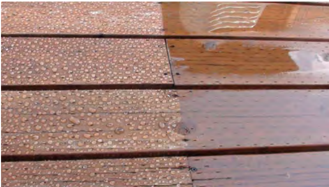
Picture 93 - Rainwater droplets on SurfaPaint Wood Stain treated deck (left), in contrast to conventional wood stain treated surface (right).
