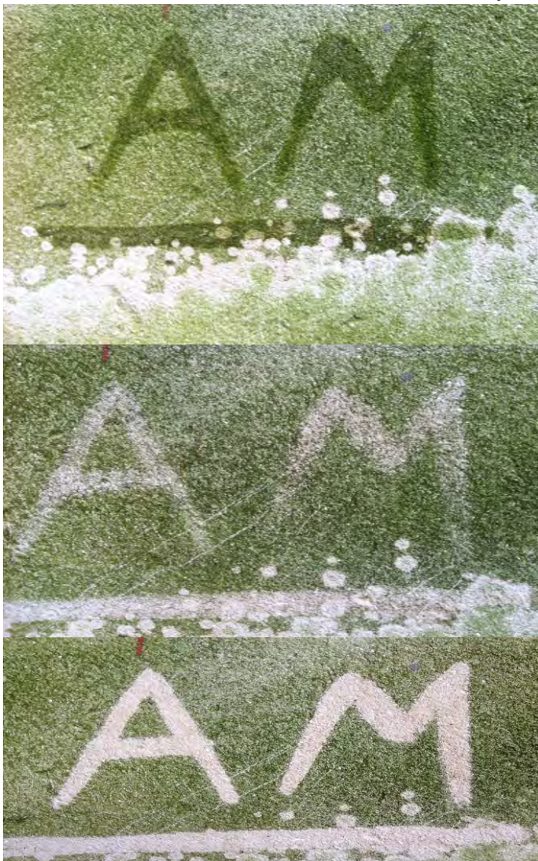
Picture 19 - The application of DeSalin AM on a mouldy surface, immediately, after 24h and after 10days from application
