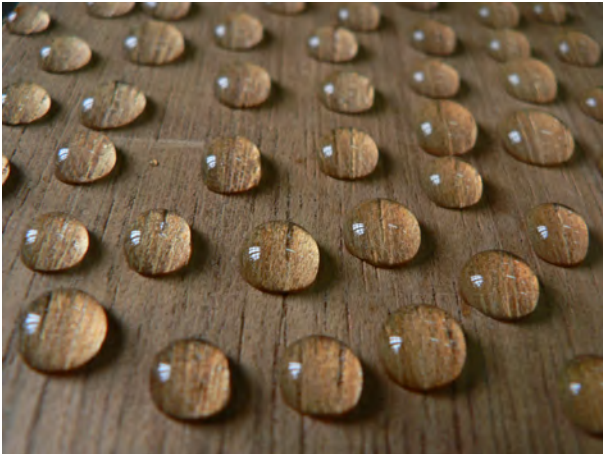
Picture 54 - Application of SurfaPore W on natural wood deck
