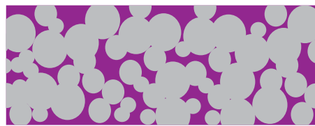
Picture 104 - Depiction of how SurfaMix C works: Cementitious materials require water for bonding and hardening. Uncontrolled setting can induce cracking of the surface or extended capillaries formation (left side). SurfaMix C controls the water reaction with cementitious materials, decreasing rapid shrinkage and cracking. At the same time, a bonding grid fills the microscopic gaps, enhances the elasticity of the material and promotes bonding on the application surface (right side).
