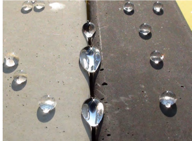
Picture 12 - The beading effect on grout is intense, even if the grout gap is huge
