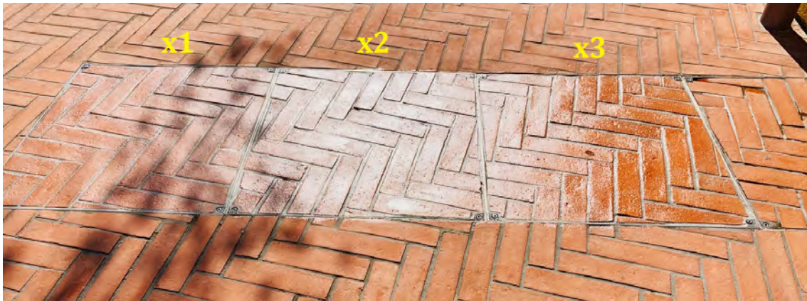
Picture 86 – Application of SurfaPaint Stone Varnish WB on cotto floor tiles, which have the same porosity structure as natural stones. Numbers depict how many coats were applied. The gloss effect gradient is clearly visible.
