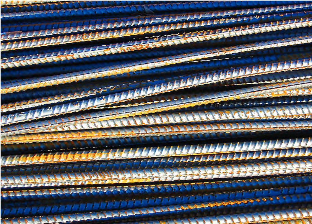
Picture 109 – Steel bars need corrosion inhibitors to prevent corrosion development before installed in cement base
