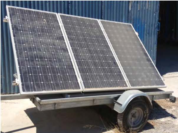
Picture 26 – Anti-dust performance of SurfaShield G coated panels: Two left panels have been treated with SurfaShield G, while the right one remains untreated for six months in Cyprus. Note the accumulation of dust in the aluminium base of the panels
